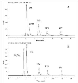
Figure 2. Chromatograms of standard drug mixture samples, without Na<sub>2</sub>SO<sub>3</sub> in the mobile phase; 140 mg/L MTZ, 80 mg/L TMD, 40 mg/L ROP, and 40 mg/L BUP (A); and adding Na<sub>2</sub>SO<sub>3</sub> (0.5 mg/mL) in the mobile phase; 100 mg/L MTZ, 30 mg/L TMD, 20 mg/L ROP, and 20 mg/L BUP (B).
